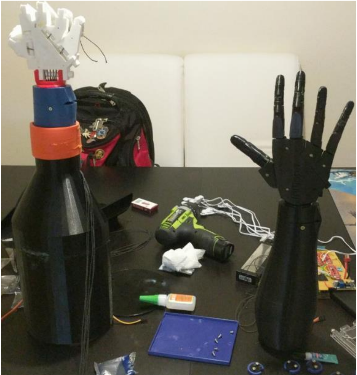
Figure 3.16: Designed forearm on the left and InMoov forearm to the right.
