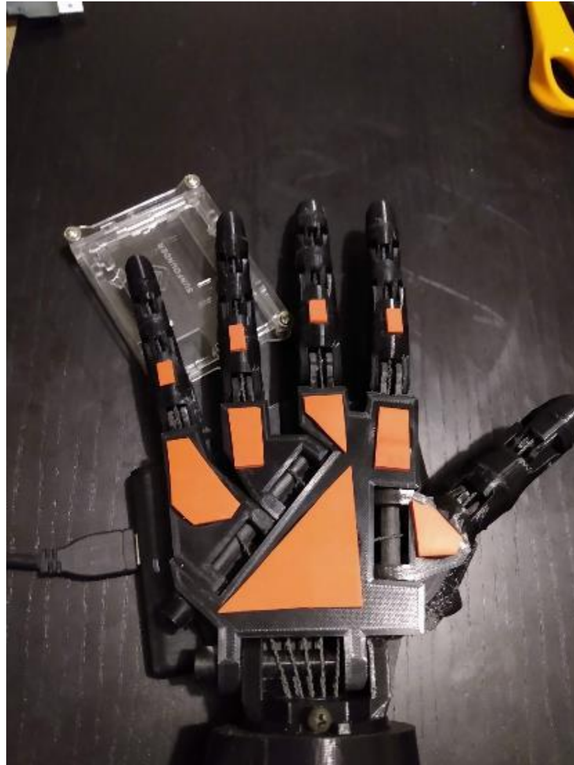
Figure 3.23: Rubber paddings for better gripping.
