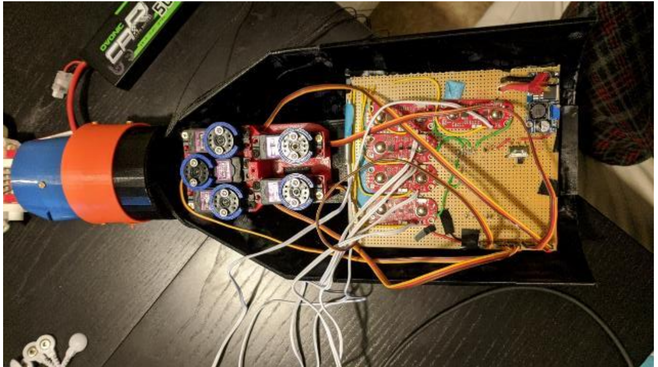
Figure 3.14: Circuit board and servo motor pulleys in new forearm.
