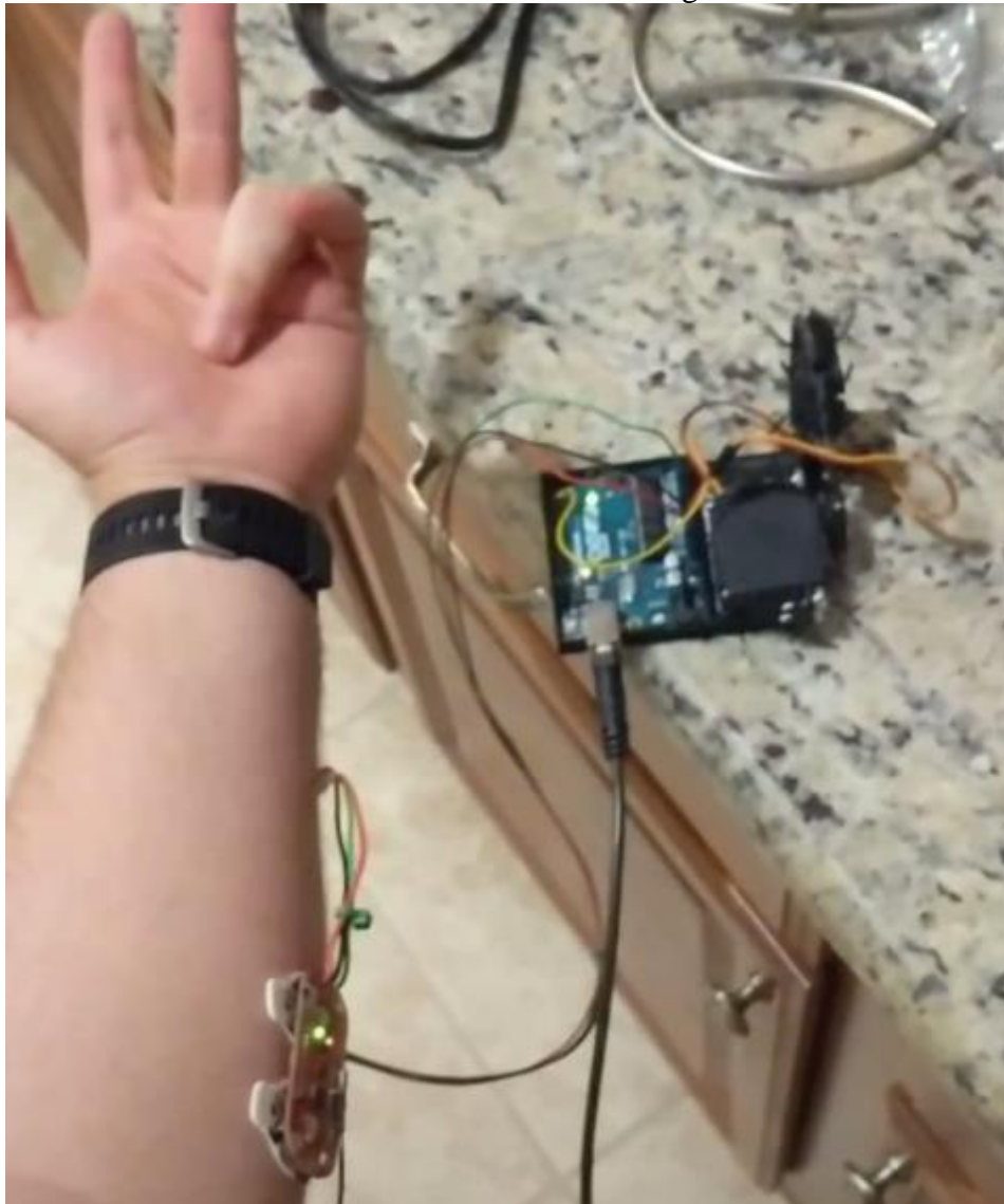
Figure 3.3: Controlling Finger Starter using the MyoWare muscle sensor board.
