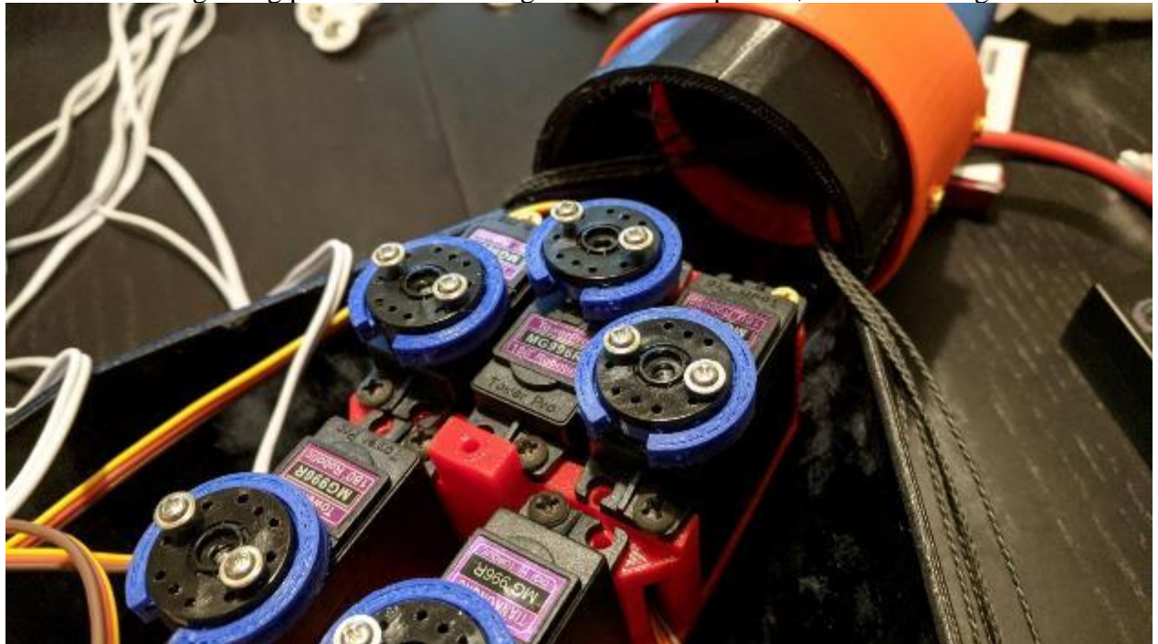
Figure 3.15: Missing fishing line guides.
