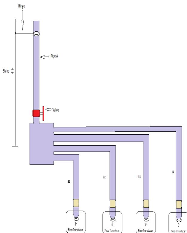
Fig. 2. Parallel operation of transducers
