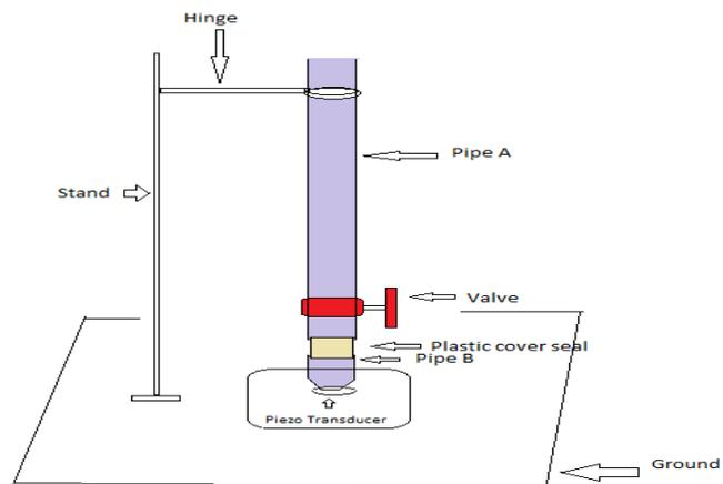
Fig. 1. Basic construction of the pipe and piezo transducer combination
