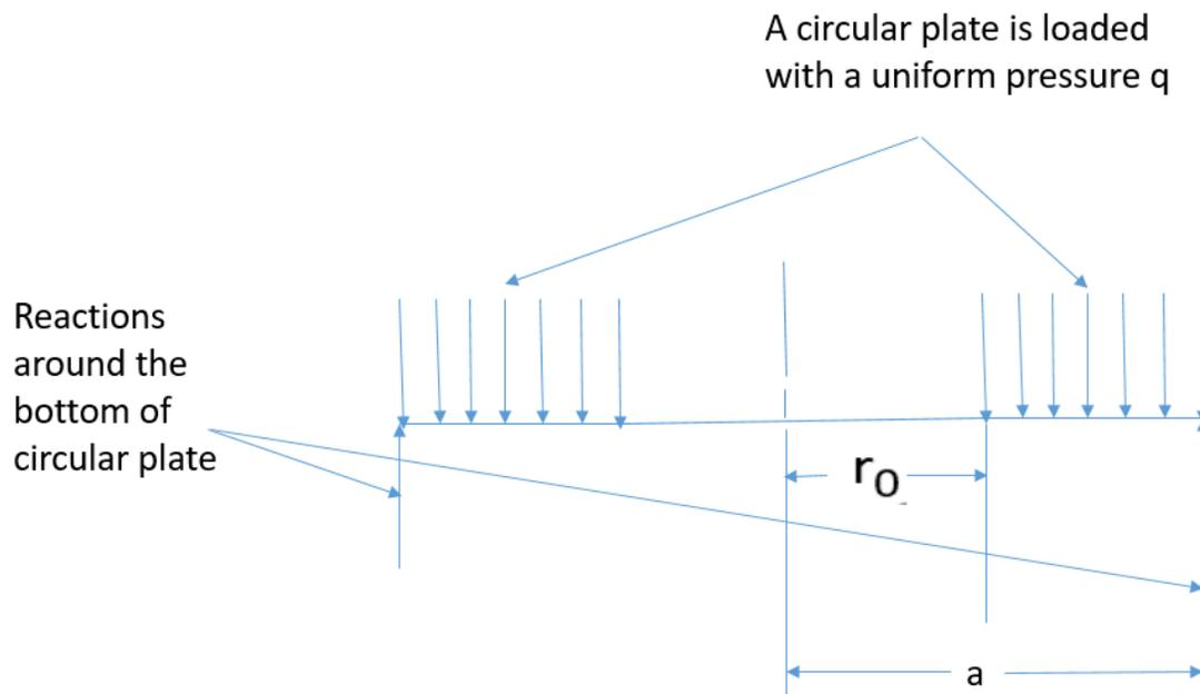
Figure 1: Side view a circular plate supported at its edge subjected to a uniformly distributed pressure
