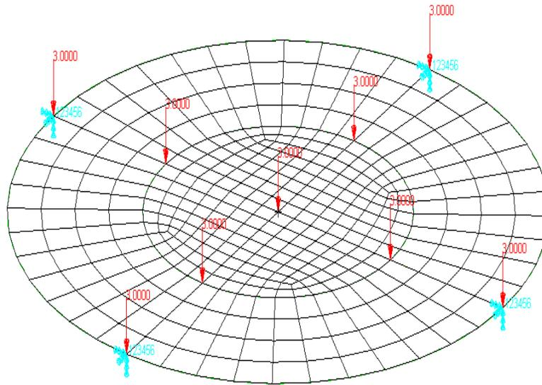
Figure 4: Finite Element Model of a 20 inch ID circular plate with a uniform thickness of 0.2 inch that is fixed at its edge and is subjected to 3 PSI uniform pressure
