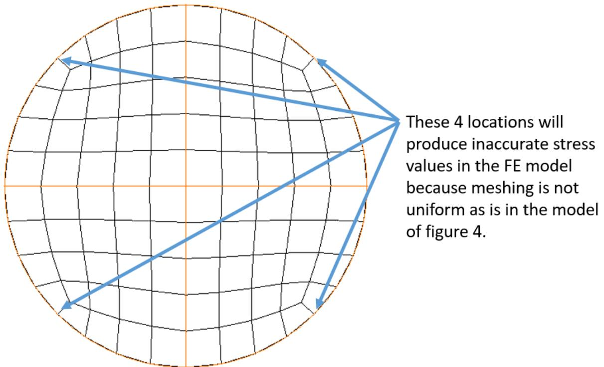
Figure 6: Demonstration of improper FE modeling practice that will result in incorrect stress values
