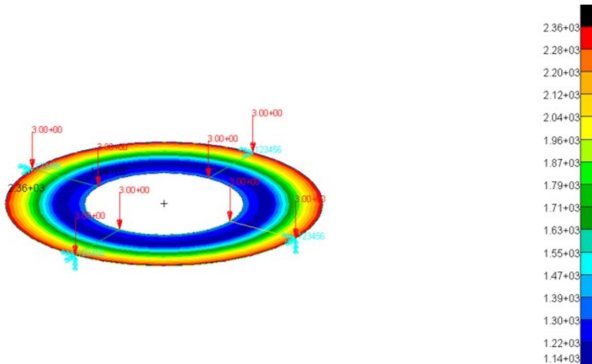
Figure 10: Stress contour of the FE model of figure 9
