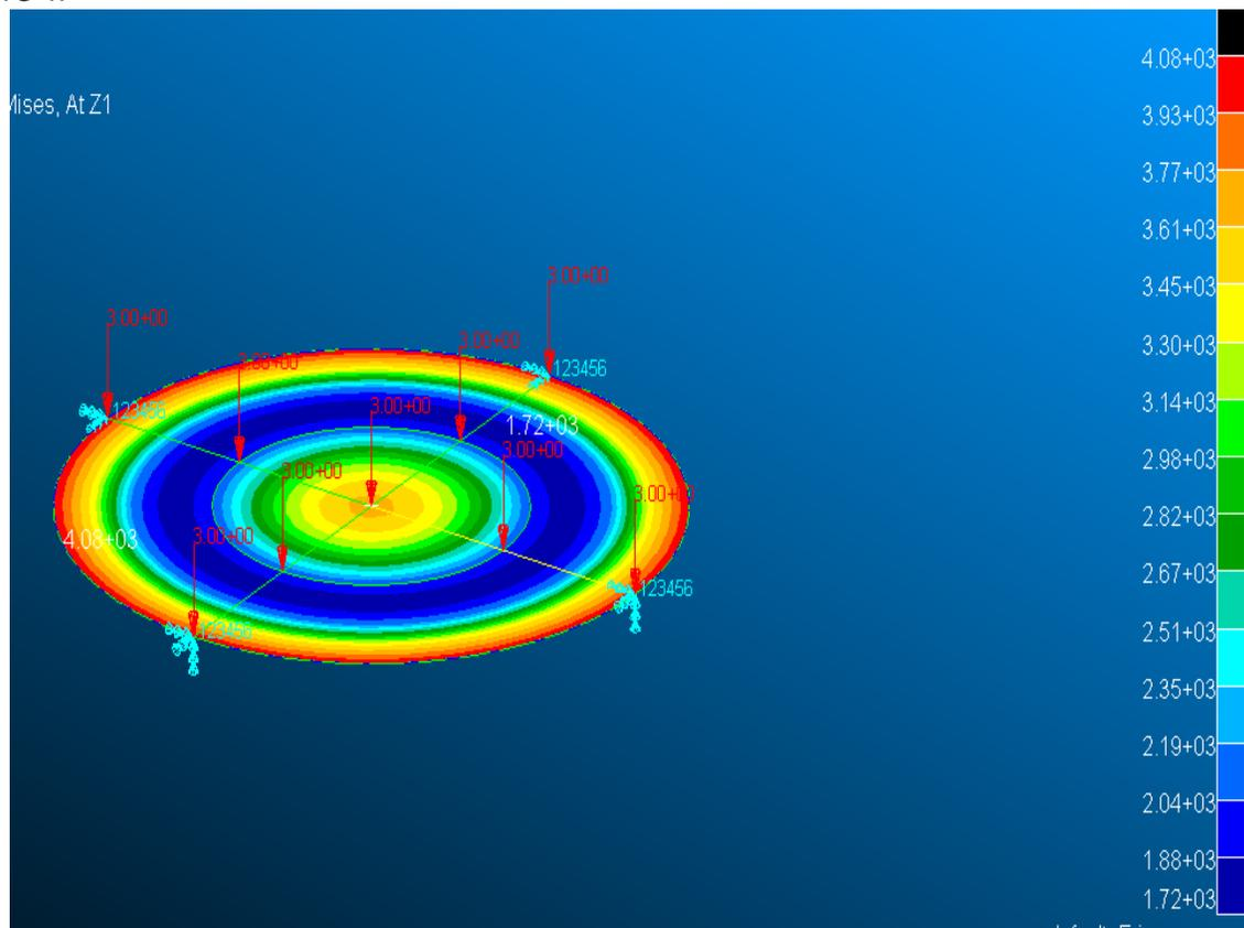
Figure 5: Finite Element stress contour obtained by NASTRAN/PATRAN for the Finite Element model of figure 4
