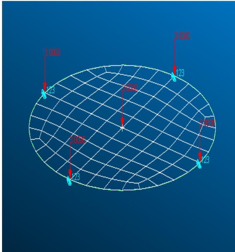
Figure 2: Finite Element Model of a 20 inch ID circular plate with a uniform thickness of 0.2 inches that is simply supported at its edge and is subjected to 3 PSI uniform pressure
