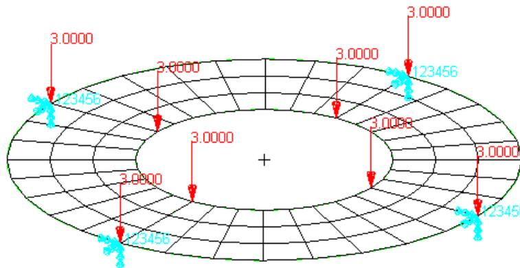
Figure 9: FE model of the model of figure 4 where a centric hole is added
