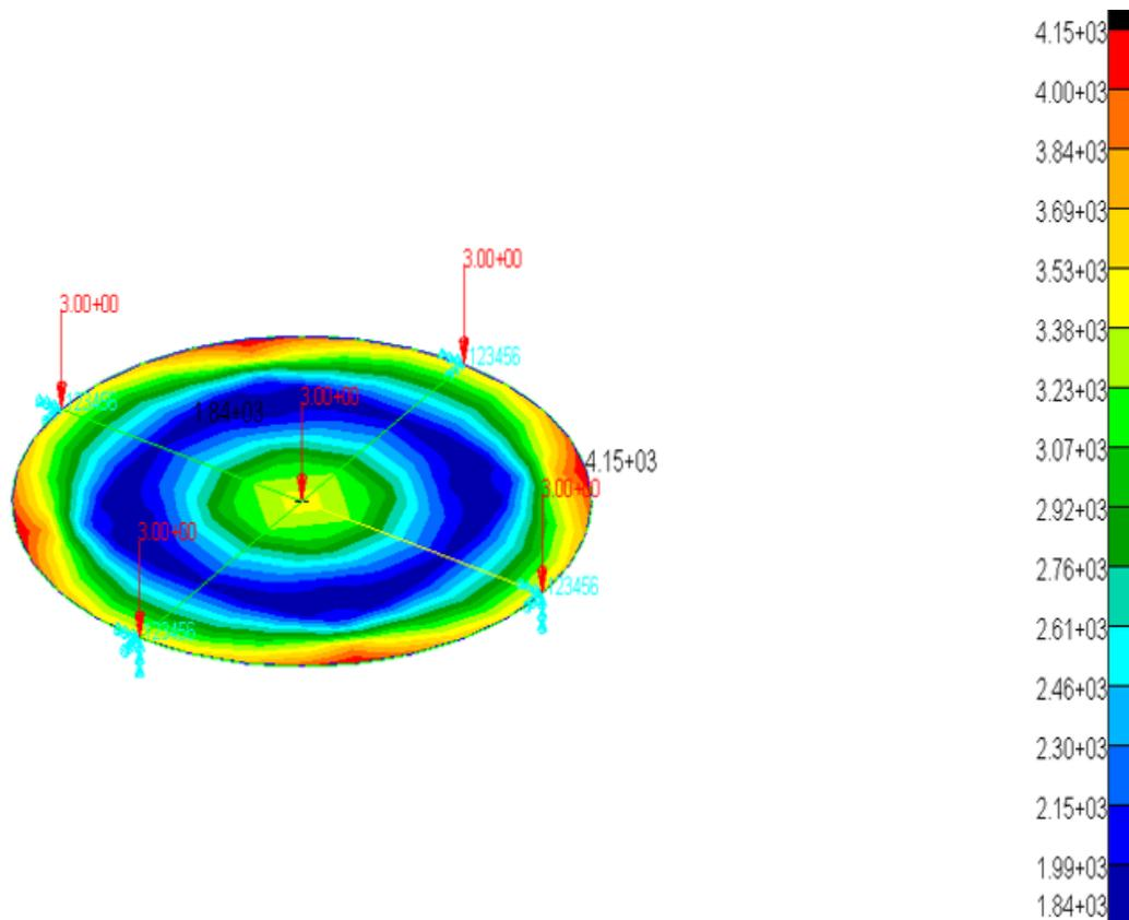
Figure 7: Stress contour for a FE model with conditions of the model of figure 4 but with improper meshing of figure 6
