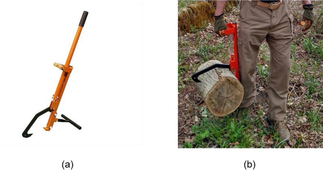
Fig. 1. (a) LogOX 3-in-Forestry MultiTool and (b) Tool in Log Hauler Configuration
